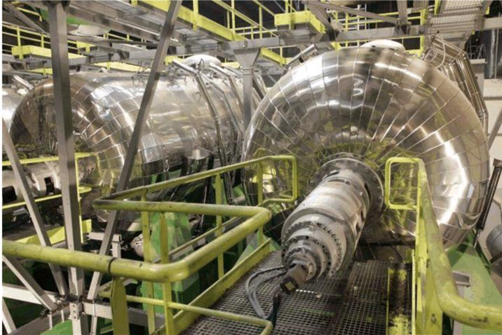
Photo: Two autoclaves in the Polish Bioelektra recycle facility where household waste is processed and recycled. (Supplied: Bioelektra)
