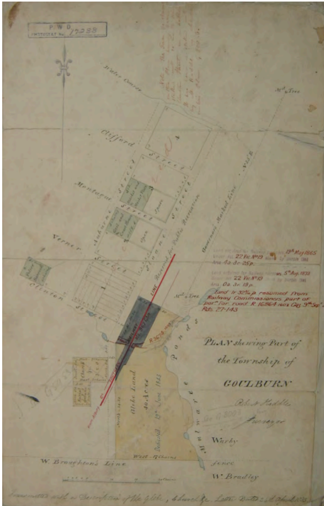
Figure 7.5. Plan showing part of the Township of Goulburn. Originally surveyed in April 1833, this plan is important as the added information shows how the railway was to cut across the southern end of Sloane Street, causing its realignment after 1869. Source. R Hoddle, Apr 1833, SR Map 1848.
