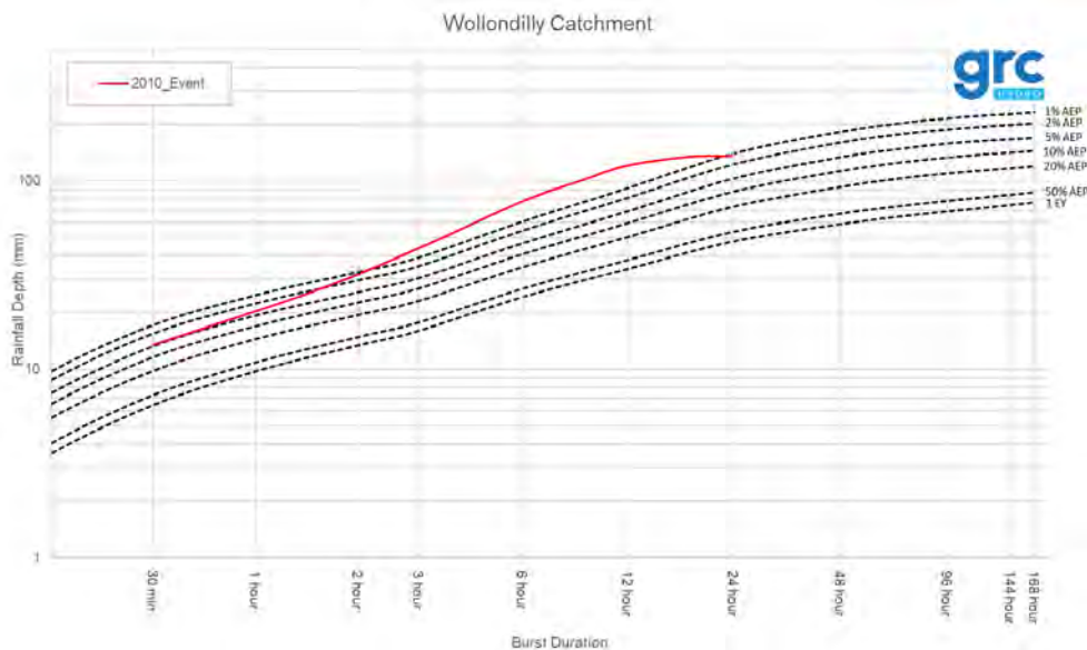
Image 4: Wollondilly River catchment – 2010 event storm burst comparison to ARR2016 IFD relationships
