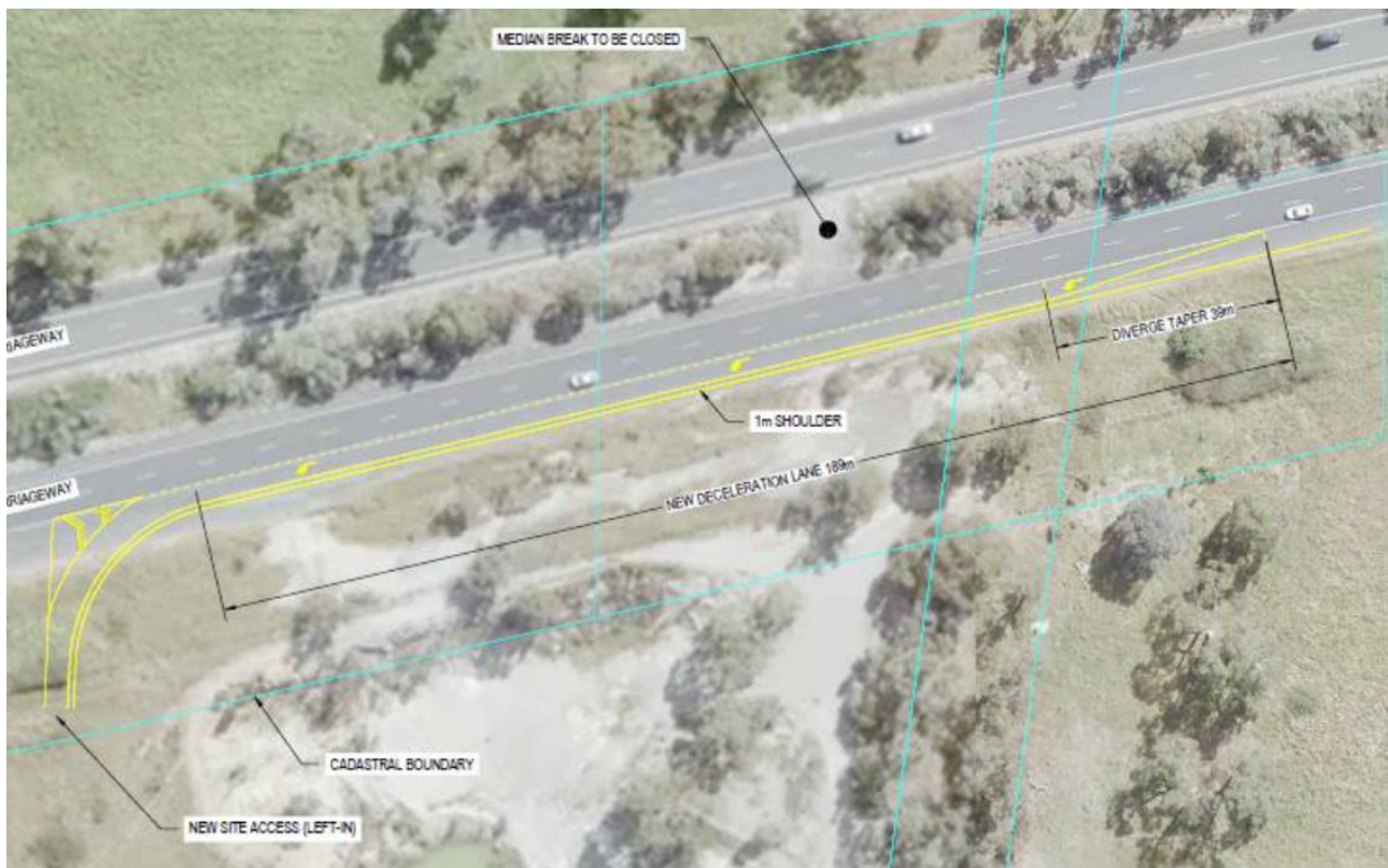
Figure 4 – New Quarry Intersection
