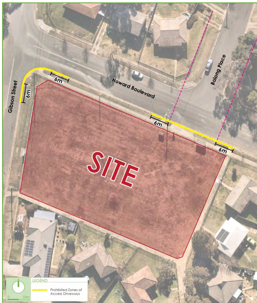
Figure 10: Prohibited Zones of Access Driveways
