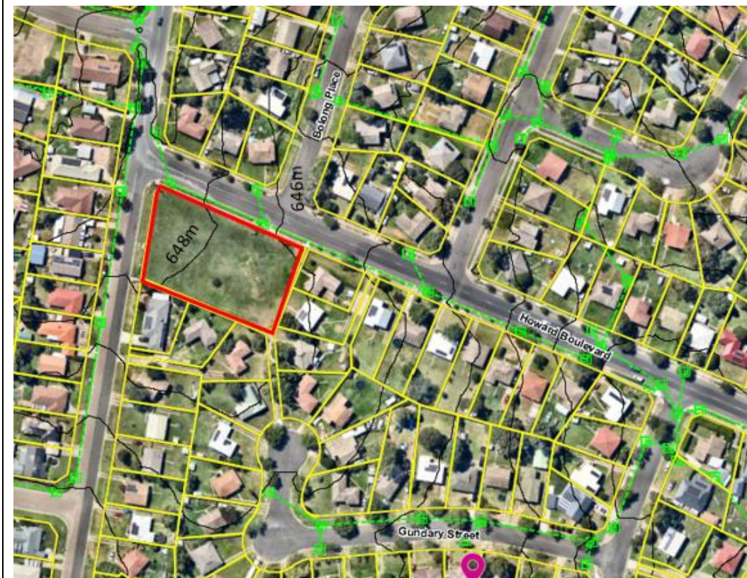
Figure 7 - Street drainage network and 2m contours.
