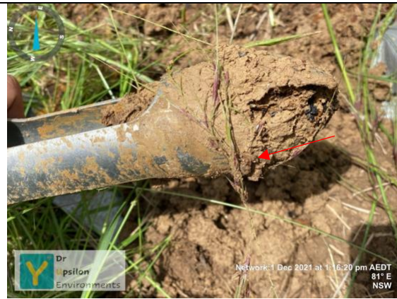
BH05_0.4; Clay with gravel, brown, moist. Results: Negative.
